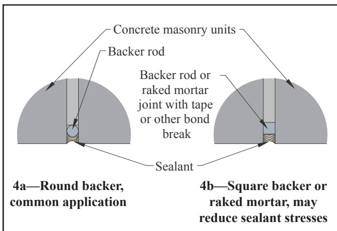
**Figure 4—Detail of Control Joint Surface (ref. 6)**
